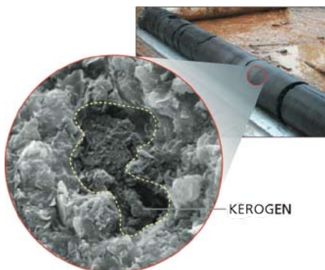
FIGURE 3-20. Shale Core, with Scanning Electron Micrograph indicating Kerogen Content
