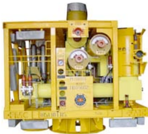
Figure VA3.1. Existing HPHT subsea tree rated to 15,000 psi and 350°F.
